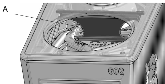
Fig. 28 Replacing the exhaust reflector
